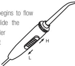
Lowest position allows you to pause completely the water flow
